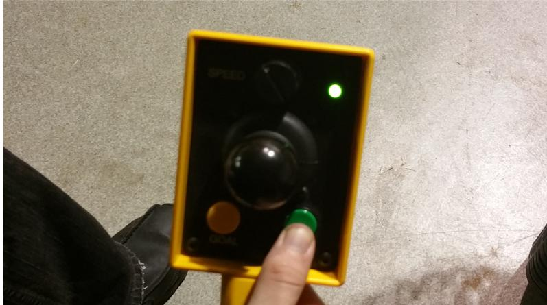
Figure 6: Joystick active and ready for movement
