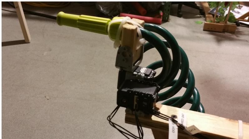
Figure 12: Servos and spraying apparatus
