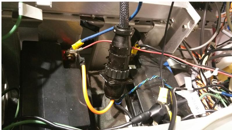
Figure 4: Batteries and main robot power connector
