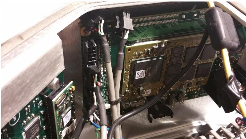
Figure 7: Location of RS-232 data connection to robot base
