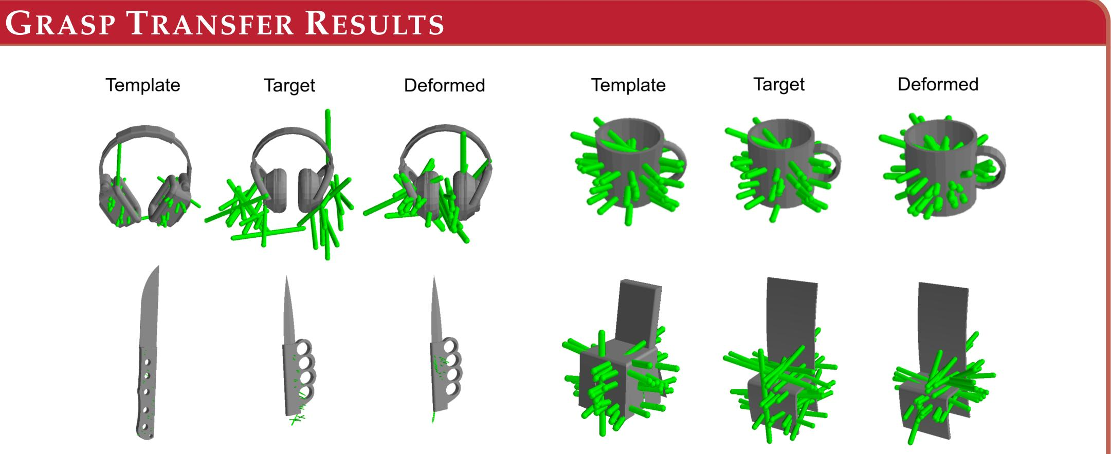
Transfer of grasps (green lines) without and with deformation, respectively.
